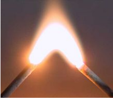
Figure 7. A continuous high current density arc-mode plasma.
